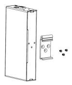
2. Insert the top of the Din-Rail clip onto the Din-Rail track, then gently push the bottom of the hub to secure it to the Din-Rail track
