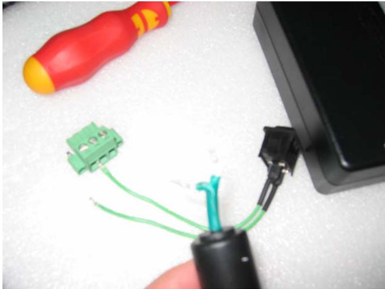
Now, screw down the first side of the power switch (ignition) in the middle of the connector.
