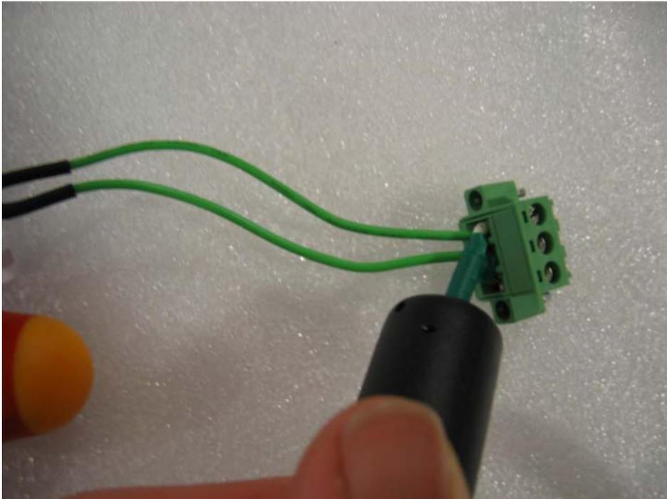
GND (grounding) has to be connected on the right side of the power connector.
