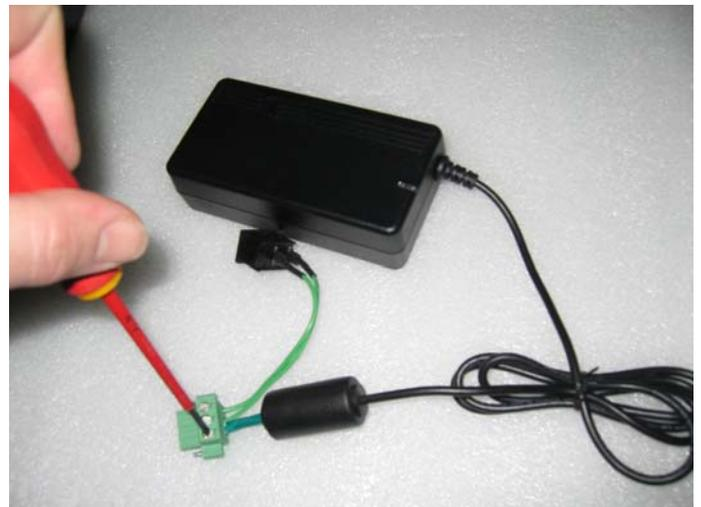
Now, +12 V and GND (grounding) have to be pulled apart slightly, because +12V and GND are on the left, and right side of the plug. (NOTE: Maybe you have to remove a little bit the isolation of the power cable.)
